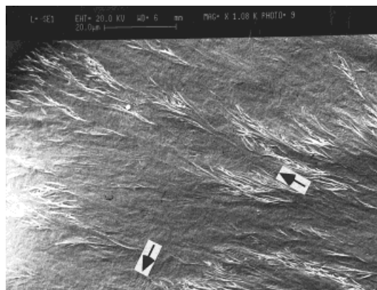
Figure 12 Scanning electron micrograph showing edge of \beta -spherulite grown at 128°C.
